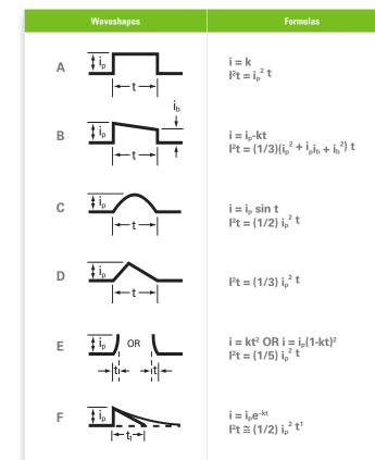
Step 3–Examine the I<sup>2</sup>t rating data for the PICO<sup>2®</sup>, 125 V, very fast-acting fuse. The part number 251001, 1-ampere design is rated at 0.256 A<sup>2</sup> Sec., which is the minimum fuse rating that will accommodate the 0.2327 A<sup>2</sup> Sec. value calculated in Step 2. This 1-ampere fuse will also accommodate the specified 0.75-ampere normal operating current, when a 25% derating factor is applied to the 1-ampere rating, as previously described.
