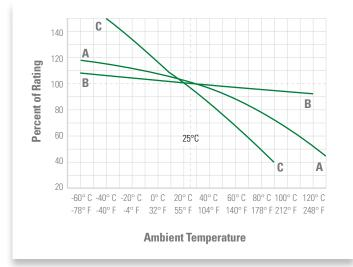
Curve A: Thin-Film Fuses and 313 Series (.010 to .150 A)
