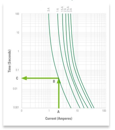
This nominal melting l<sup>2</sup>t is not only a constant value for each fuse element design, but it is also independent of temperature and voltage. Most often, the nominal melting l<sup>2</sup>t method of fuse selection is applied to those applications in which the fuse must sustain large current pulses of a short duration. These high-energy currents are common in many applications and are critical to the design analysis.
