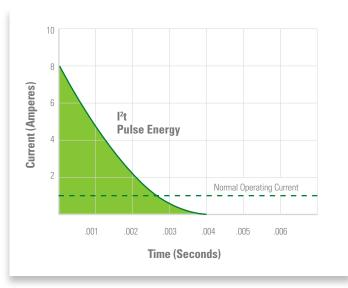
Step 2–Determine the required value of Nominal Melting I<sup>2</sup>t by referring to the <u>Pulse Cycle Withstand Chart</u>. A value of 22% is shown for 100,000 occurrences of the Pulse I<sup>2</sup>t calculated in Step 1. This Pulse I<sup>2</sup>t is converted to its required value of Nominal Melting I<sup>2</sup>t as follows:
